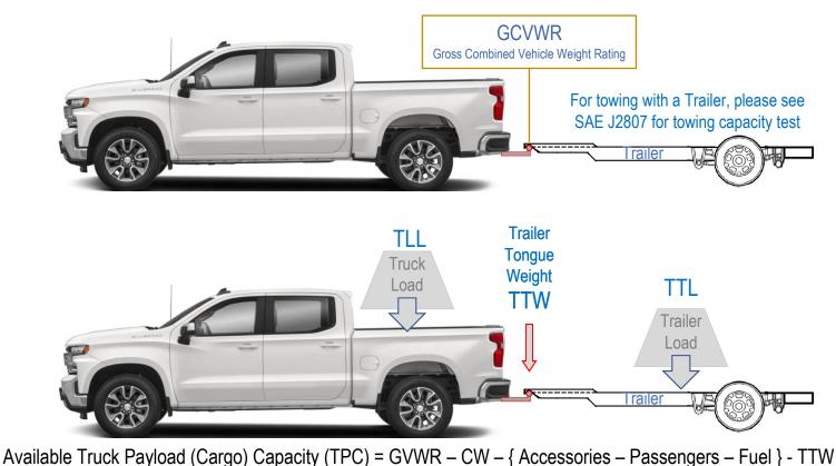
Available Truck Payload (Cargo) Capacity (TPC) = GVWR – CW – { Accessories – Passengers – Fuel } - TTW
