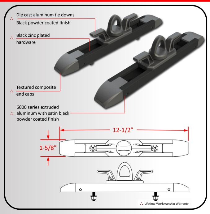
These Cargo rails from ApexOEM are the perfect way to secure your gear. This patented design is made with lightweight 6000 series aluminum and is compatible with standard 1-5/8" channel hardware. A black powder coated finish offers durability and a great look.
